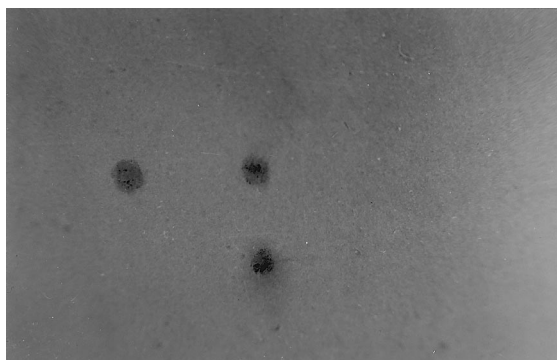
Fig. 3. Photograph of an actual chromatogram showing resolution of DL-lysine, as typical results. Left to right: (1) pure L-lysine; (2) resolved DL-lysine. Temperature, 26 \pm 2^\circ\text{C} ; solvent front, 8.5 cm; detection, ninhydrin; solvent system, acetonitrile-methanol-water (10:5:2 v/v).
